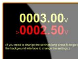
Lowvoltage alarm interface
