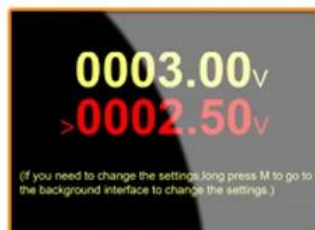
Low-voltage alarm interface
