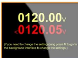
Over-voltage alarm interface
